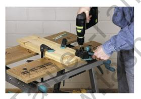
The universal and quick dowelling jig for corner, T-butt and edge-to-edge connections
